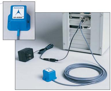
**3D-BIRD,** shown with its power supply, connects directly to the RS-232 serial port of your host computer. Sensor data is processed by our driver residing on your computer.
