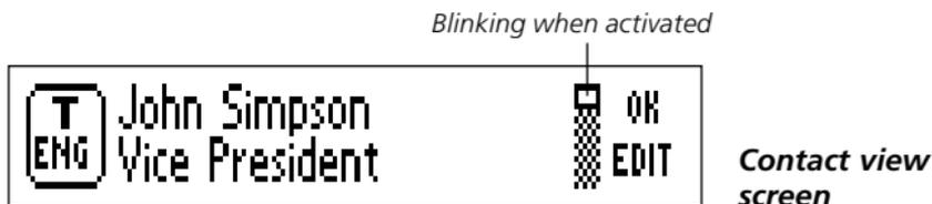
To select **OK** or **EDIT**, first press **Nav** to deactivate the scroll bar – the rectangle stops blinking – then turn **Nav** to go to the buttons.
