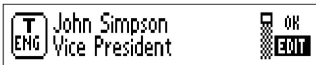
In both cases the **Contact edit screen** will open, displaying the stored information in the fields. You can move between the fields by turning **Nav**. If you want to change the content in a field, you can read a new field text with C-Pen or edit the text in the usual way.
