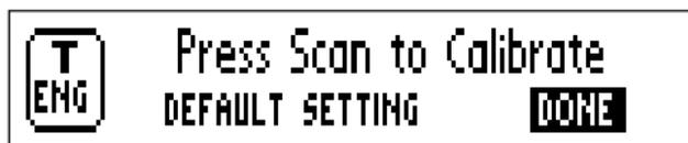
In the calibration dialog box, select **DONE** to go back or **DEFAULT SETTING** to revert to the factory setting. If you press the scan button (**Trigg**), a calibration will start.
