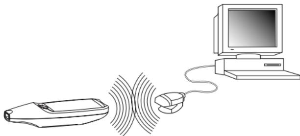
When C-Pen is within range of the computer's IR port, an IR icon will appear in the status field on C-Pen's display. On most laptops the built-in IR port - a red or black glossy square - is found on the back or side of the computer.
