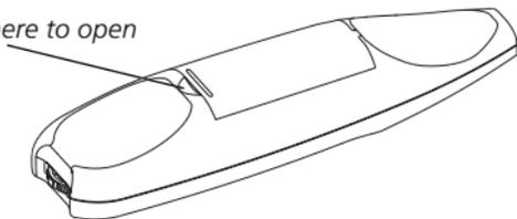
2. Insert two alkaline AAA batteries (1.5 V type LR03) as shown below.
