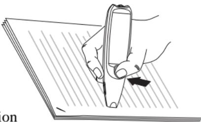
4. Move C-Pen over the line of text. Keep **Trigg** pressed as you move C-Pen over the text.
